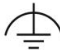
Connection of the protective equipotential bonding conductor
