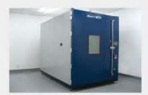
Advanced environmental test chamber can do DH (85% RH, 85 C), TC200, HF test, which can verify reliability of product.
