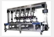
2400Pa wind load test and 5400Pa snow load test can assure the safety of solar module in the windy and snowy days.
