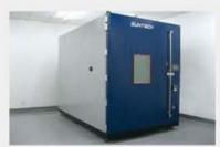
Advanced environmental test chamber can do DH (85% RH, 85 C), TC200, HF test, which can verify reliability of product.
